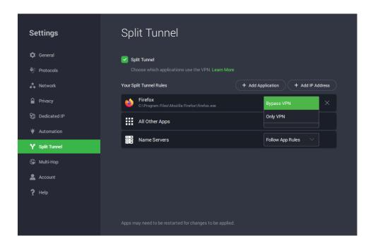
If an app is selected to bypass the VPN, that application will operate normally whether the VPN is connected or disconnected.
